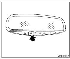
Using both hands, simultaneously press and hold both the HomeLink® button you want to program and the hand-held transmitter button.
